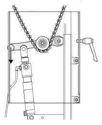
Move the tensioner downward until the chain is tightly secured in its position. There should be a gap of about 12.7 mm between the pneumatic-piston nut and pneumatic piston, where the piston should be visible.
