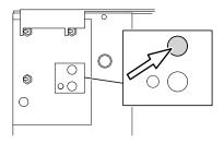
If the top-plate angles are not the same (for example 26° in the right direction and 30° in the left direction), adjust the nuts (A) a 1/2-turn at the time.
