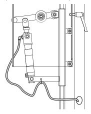
Now attach the chain holders that will allow you to keep loops of chain up off of the ground. Insert the provided long bolts into the holes located on both sides of the stand and fix them in place with a 13 mm wrench.
