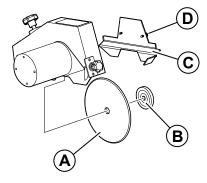
Remove the wheel attachment nut from the hub.
