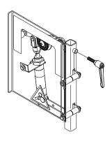
Then insert the rod through the unit and insert the bottom part of the rod onto the base of the stand
