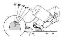
Change the grinding setting for the height of the depth gauges.
