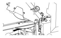
If required: Turn the chain pusher adjustment to make minor adjustments for the grinding length.
