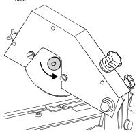
Next, insert the appropriate wheel onto the hub and, using moderate pressure with your hands, secure the wheel attachment nut to hold the wheel in place.
