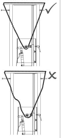
If the chain tension is too loose, repeat the procedure.
