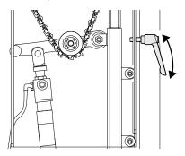
Lift the tensioner arm (there is a quick release function) and place the chain below the tensioner roll.
