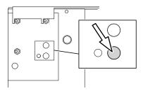
Press the grinding head positioning button to turn the grinding head to the left.
