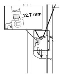
Tighten the locking handle to secure the chain.
