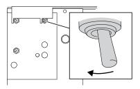
Set the chain pusher switch to ON to start the feeding of the chain and the movement of the grinding head. The sharpening will start after
