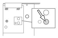
Set the grinding wheel switch to ON.
