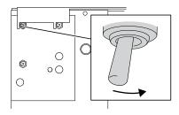
IMPORTANT If the chain has double cutters. pull the chain back so that the grinding starts on the second double cutter. If the chain has a joint with an irregular cutter sequence, start grinding behind it, to the left of the stop clamp.
