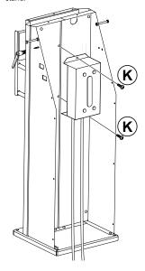
Next, place the machine on the stand. Fix it to the stand through the 3 holes located at the back and front of the machine with the bolts and nuts provided.
