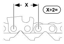
Loosen the chain pitch wing-nut and move it to the correct pitch position. Tighten it again.
