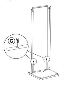
4. Next, attach the two side pieces to each other with provided bolts through the holes at the intersection of two pieces to create the side support piece.
