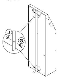
To complete the assembly of the stand, bolt the side support first to the base and then to the front piece.
