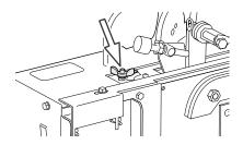
Note: Adjusting the pitch is not the same thing as adjusting the cutting tooth length (see section 5.2.7, "Set the cutter top plate to equal lengths").
