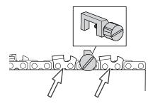
Place the chain, with the cutter to the left of the depth gauge, into the groove on the chain vise.
