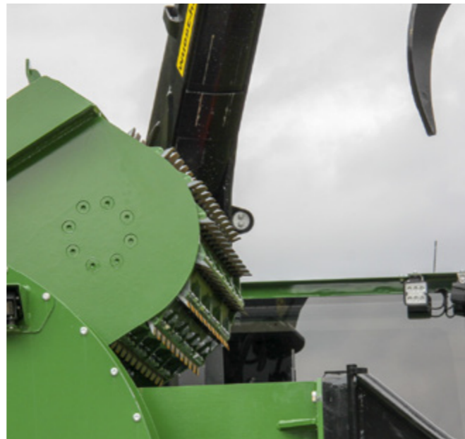
Upper infeed roll with interchangeable blades
