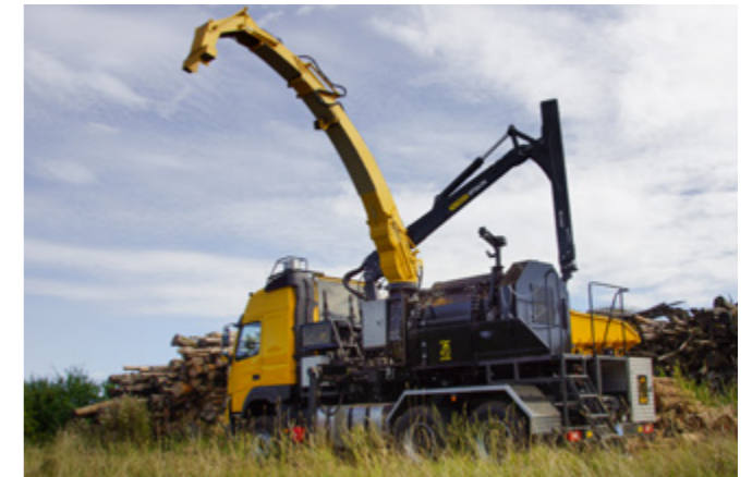
Volvo FMX, 540 PS with SMC-812, hydraulically driven accelerator, centrally arranged ejector spout
