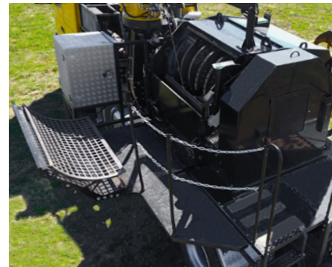
Maintenance platform with hydraulic folding
