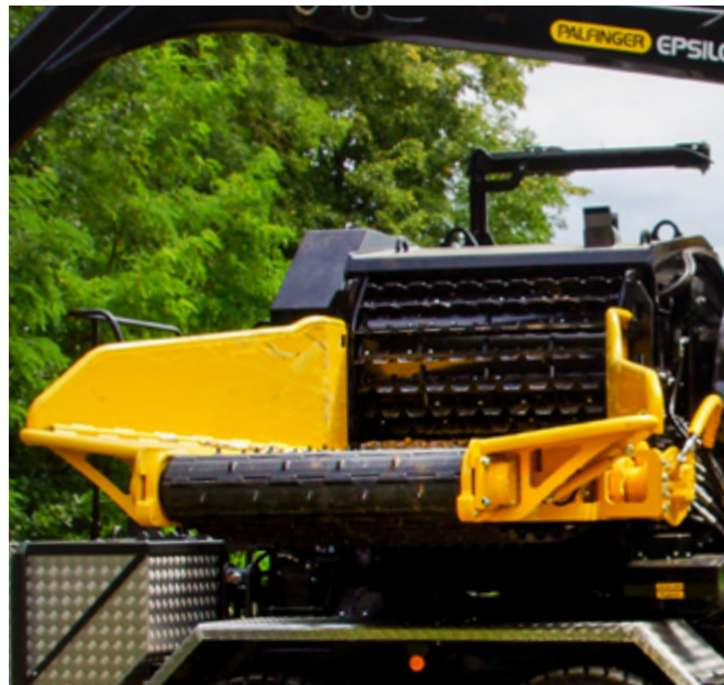
The infeed table is fitted with folding side walls to save space.
