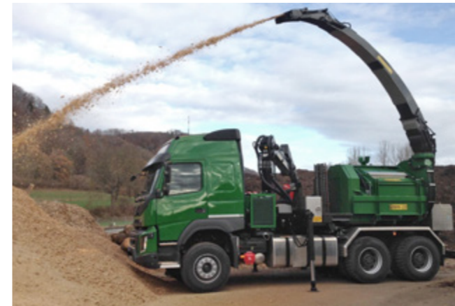
Volvo FMX, 540 HP with BBHK-120, mechanically driven fan, ejector spout arranged at the rear
